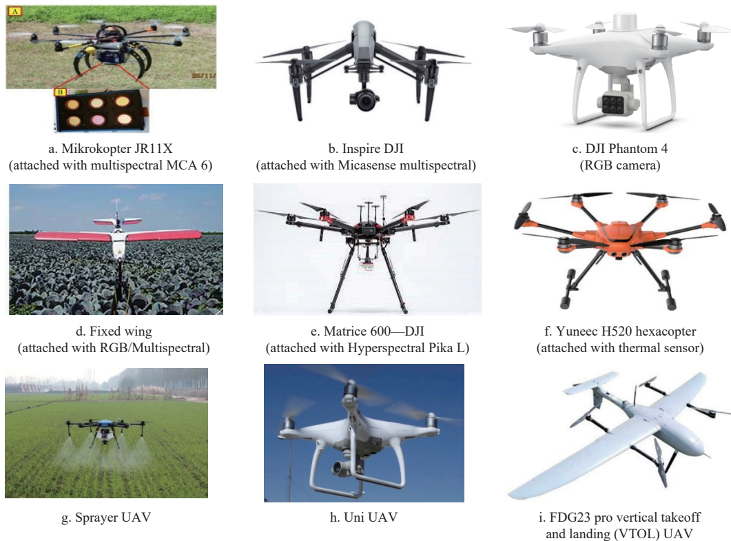
Figure 9 UAV used for classification of weed or weed and crop
