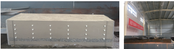
Figure 3 Experimental model of water drainage technology of the concealed pipe
