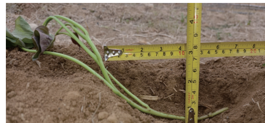
Figure 17 Transplanting track of the ship-shaped transplanting mechanism
