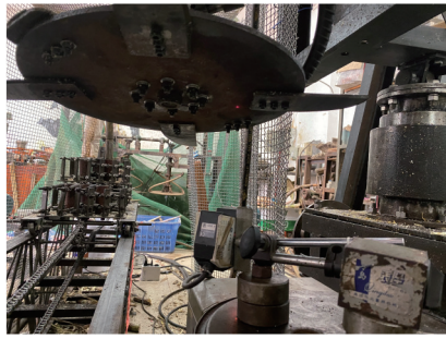
a. The laser of the LK-G150 laser displacement sensor falling on the cutter along the z axis to measure the axial cutter vibration amplitude
