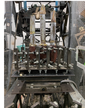
e. Piezoelectric three-directional force measuring instrument installed under the sugarcane-holding device
