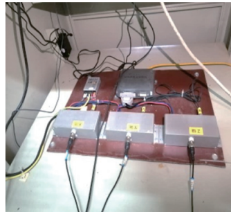
d. Three channels of the piezoelectric three-directional force measuring instrument corresponding to the x, the y and the z axes
