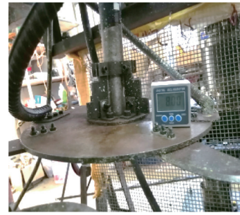
b. The digital angle-measuring instrument put on the cutter to measure the cutter inclination angle
