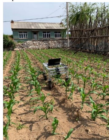
Figure 7 Experimental scenario with the fused device of camera and Lidar
