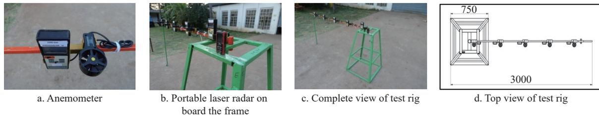
Figure 4 The developed test rig for measuring multi rotor UAV downwash airflow
