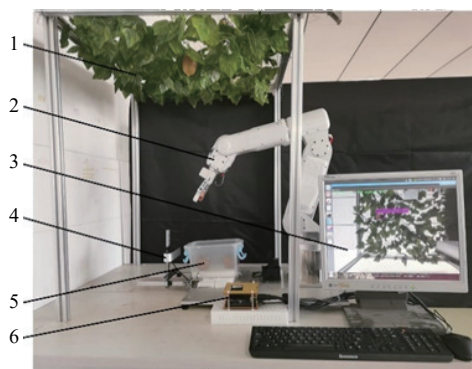
Note: 1. Indoor kiwifruits scaffolding; 2. S6H4D Plus six-axis manipulator; 3. Identification interface; 4. ZED binocular stereo camera; 5. Collection box; 6. Jetson Xavier NX system a. Indoor picking experiment
