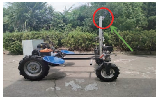
Figure 1 Camera installation location
