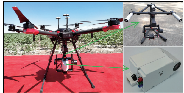
Note: Left: DJI Matrice 600 Pro UAV systems; Right: DJI Ronin-MX gimbal and Rikola hyperspectral imager.
