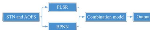
Note: STN: Soil total nitrogen; AOFS: Artificial olfactory feature space; PLSR: least squares regression algorithm; BPNN: Back-propagation neural network.
