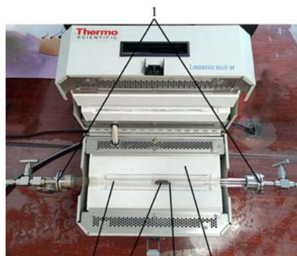
1. Vacuum flange 2. Quartz tube 3. Soil sample 4. Quartz boat 5. Pyrolysis furnace
