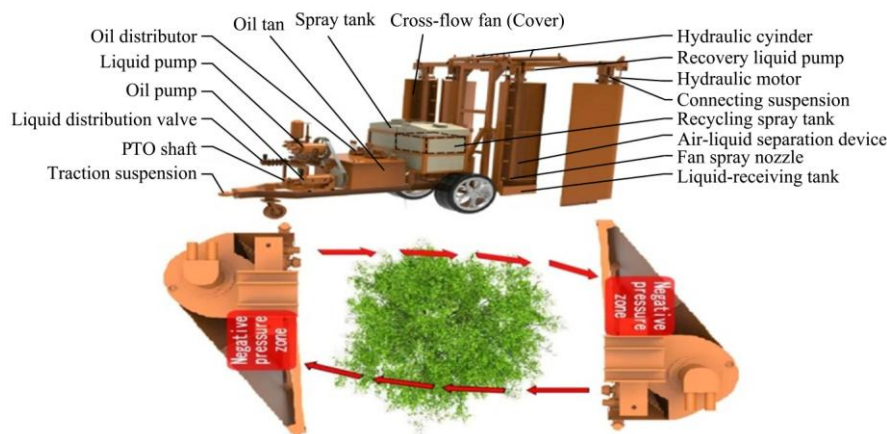
Figure 1 Structure of the tunnel-convective air-assisted atomizer
