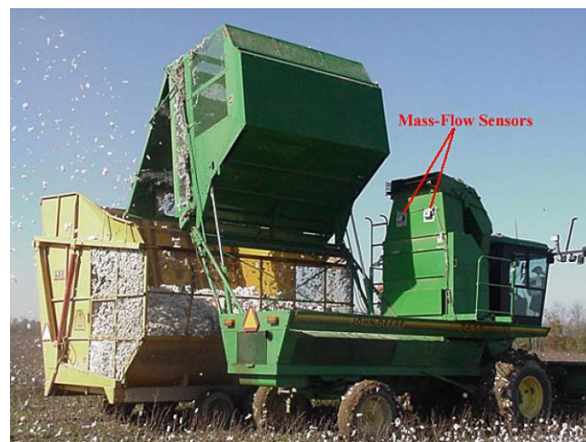
Figure 8 Two mass-flow sensors installed in a cotton stripper harvester
