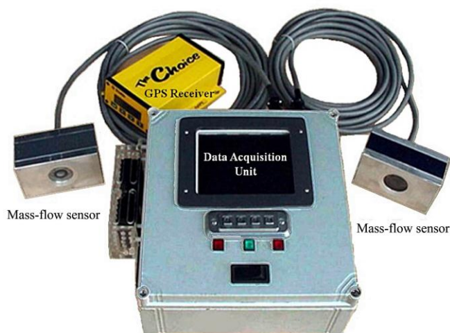
Figure 6 Mississippi cotton yield monitor including mass-flow sensors, a data acquisition unit, and a GPS receiver
