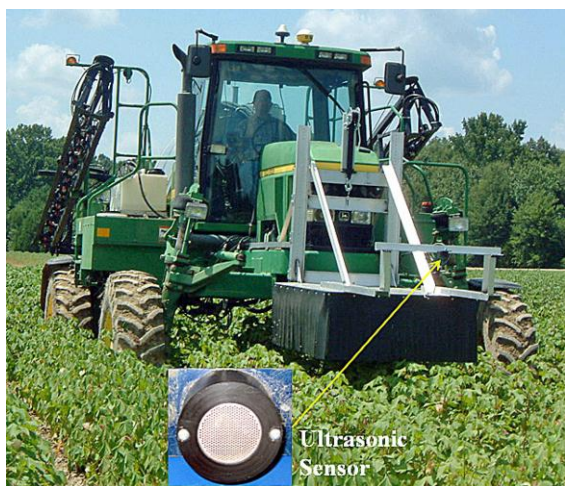
Figure 1 Ultrasonic PHMS installed in a tractor was conducting plant height measurement in a cotton field
