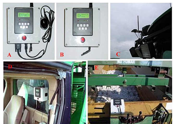
Figure 12 Wireless cotton module tracking system: (A) harvester subsystem (HS), (B) module builder subsystem (MBS), (C) wireless antenna of HS on top of the picker's light bar to enhance wireless transmission, (D) installation of HS in the cab of a cotton picker, (E) installation of MBS on a module builder
