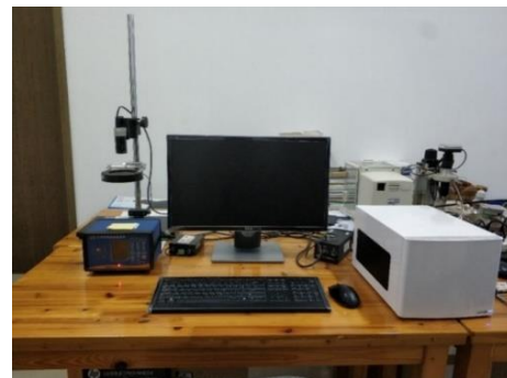
Figure 2 Point cloud data collection system
