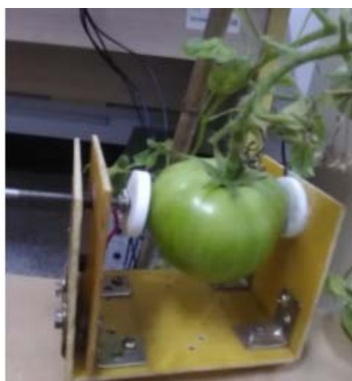
Figure 2 Experimental device for electrical impedance measurement of tomato fruit
