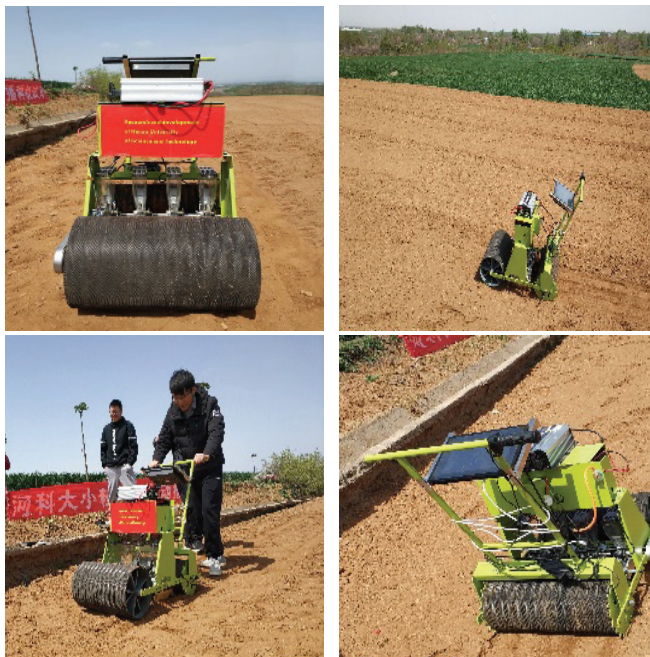
Figure 10 Field test of electric seeder for small seed
