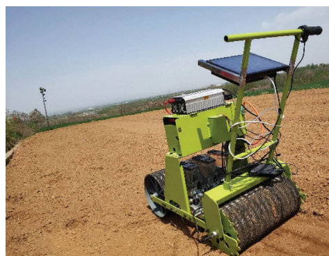
a. Overall structure sketch 1. Speed governing knob 2. Rack 3. Rear repressing wheel 4. Power supply box 5. Seeder 6. Front pressing wheel 7. Ditching device 8. Earthing device 9. Built-in drive motor
