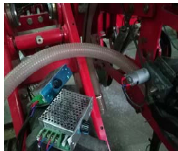
Figure 10 Speed regulator and the fan
