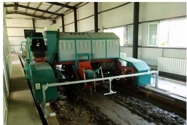
Figure 9 Ground information acquisition test bed and earth tank testing vehicle
