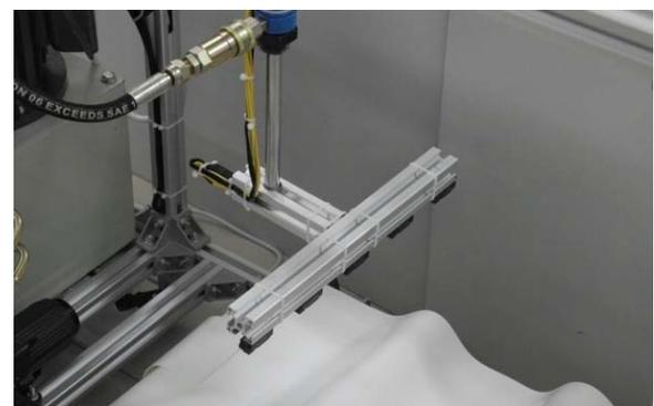
Figure 6 Infrared ranging sensor group
