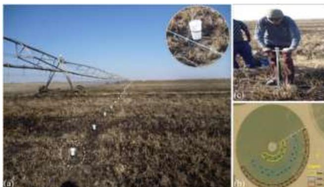
Figure 2 Field data collection: (a) setup of irrigation performance test, (b) soil samples allocation and (c) soil samples collection
