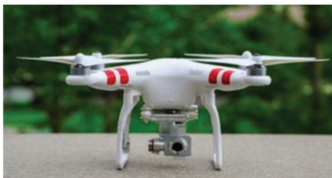
Figure 2 Image showing the DJI Phantom 2 Vision+ Unmanned aerial vehicle remote sensing platform used for this study with the gimbal and high resolution camera attached
