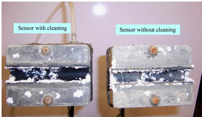
Figure 5 Photographs showing clay/silt fouling and bacterial fouling on sensors after a 40 d cleaning experiment
