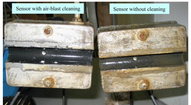
Figure 8 Aluminum sensors after working in water for 4 d
