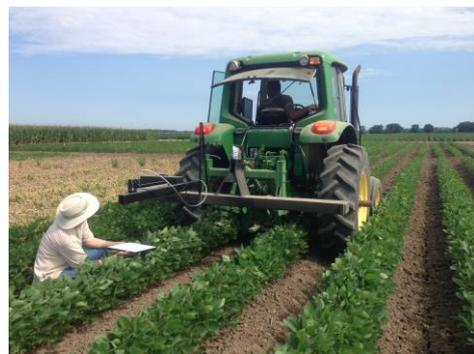
Figure 2 Field on-the-go system hyperspectral imaging system.
