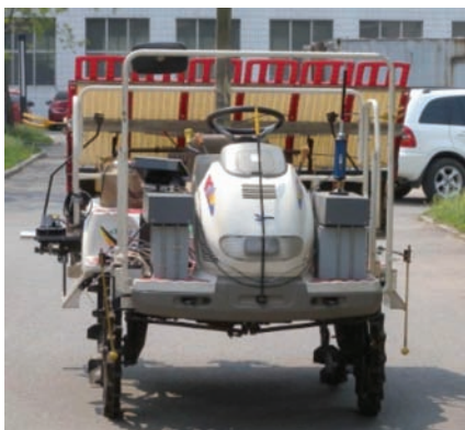
Figure 2 Rice transplanter equipped with automatic navigation system
