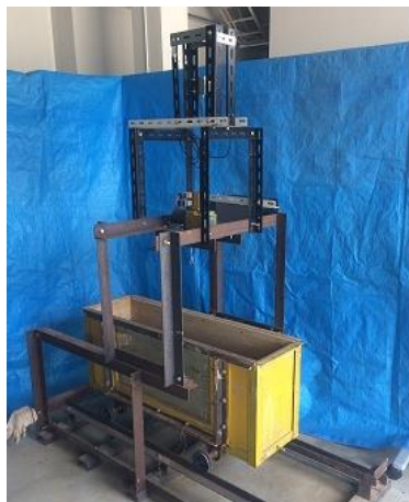
Figure 7 Locale photo of penetration tester device
