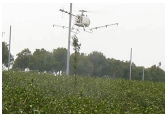
Figure 4 Spraying unmanned helicopter used for tea plantation frost protection
