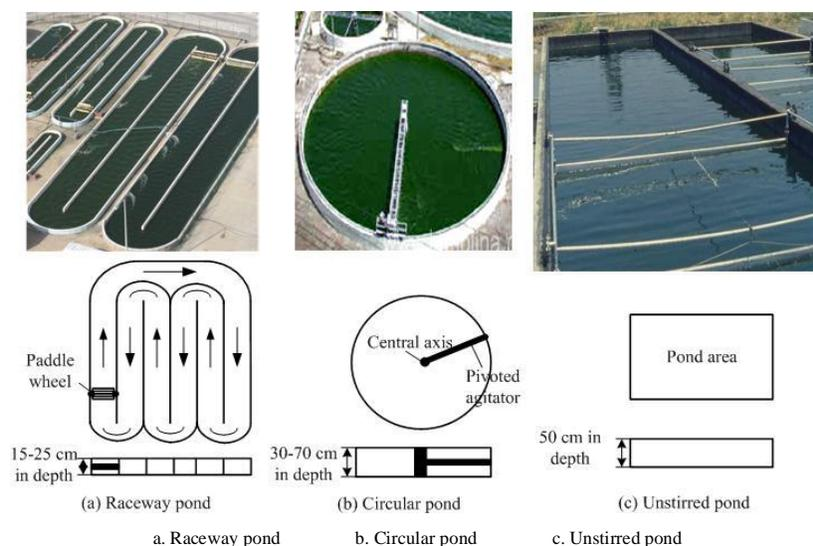
Figure 1 Three different designs of open pond systems (a and b: courtesy of A. Ben Amotz, National Institute of Oceanography, Israel; c: courtesy of M. R. Tredici<sup>[26]</sup>, University of Florence, Italy; d: courtesy of M. A. Borowitzka<sup>[27]</sup>)
