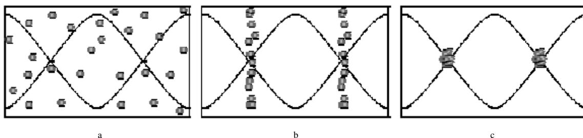
Figure 6 Principle of the ultrasonic harvesting process: When algal cells are exposed to an ultrasonic standing wave (a), they are driven to the planes of the low pressure nodes of the field (b). Subsequently, agglomeration of the cells occurs into the knots of the ultrasonic field (c). When the field is nullified, the large algae aggregates settle rapidly from the fluid due to gravity forces<sup>[66]</sup>
